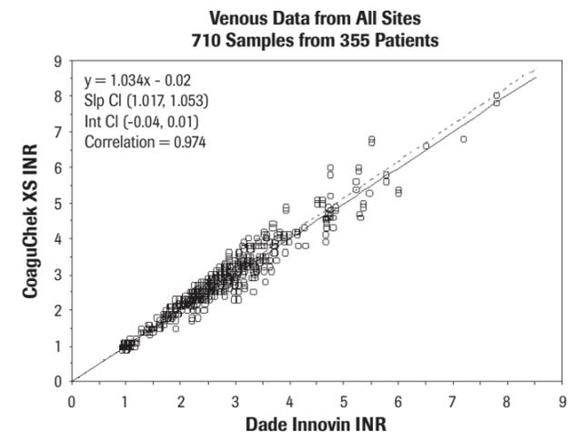
**Accuracy:** 700 capillary samples were collected from 357 outpatients at three external sites. Capillary blood samples were assayed on the CoaguChek XS meter with the CoaguChek XS PT Test and venous plasma samples were measured on a Dade Sysmex 560 Analyzer using Dade Innovin (ISI = 1.02) The results comparison is as follows:
